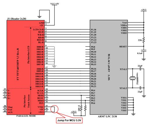
Figure 3.2A displays example of connecting Board ET-TFT240320TP-3.2 REV.B with MCU ARM7 #LPC2138(3.3V).
