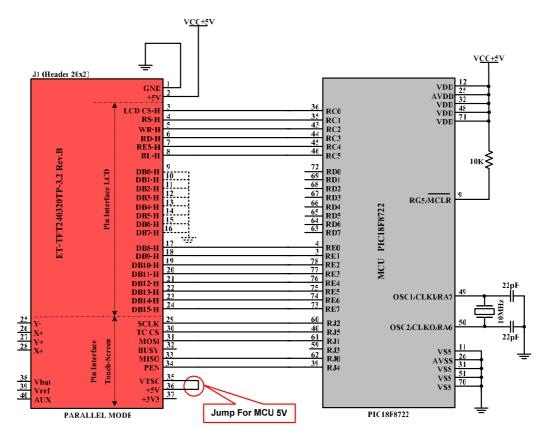
Figure 3.2C displays example of connecting Board ET-TFT240320TP-3.2 REV.B with MCU PIC #18F8722(5V).
