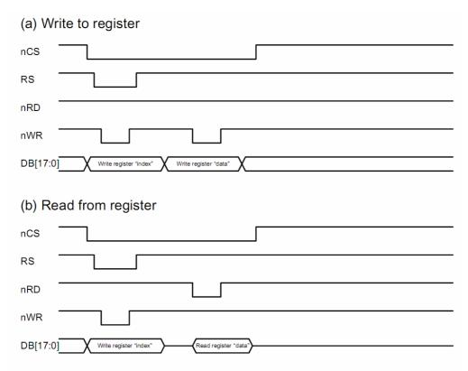
Figure 4.1.3C displays Timing Diagram to Read-Write Command and Data to LCD as Parallel 16-Bit Mode.
