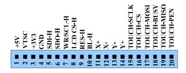
Figure 2.2 shows pin position of Header 1x20(SPI-MODE)(front view as shown in the figure 2.1(A)).
