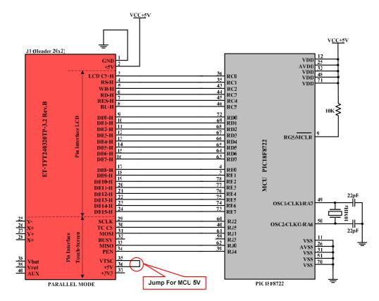
Figure 3.3C displays example of connecting Board ET-TFT240320TP-3.2 REV.B with MCU PIC #18F8722(5V).
