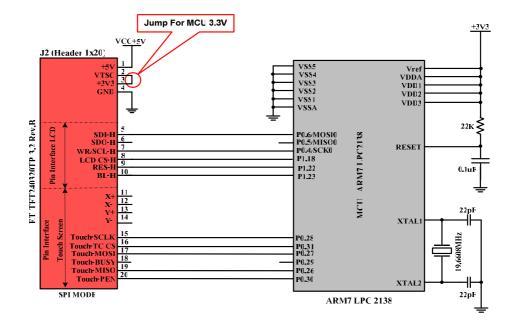
Figure 3.1A Display example of interfacing Board ET-TFT240320TP-3.2 REV.B with MCU ARM7 #LPC2138(3.3V).
