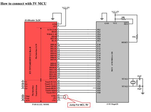
Figure 3.3B displays example of connecting Board ET-TFT240320TP-3.2 REV.B with MCU AVR #Mega128 (5V).
