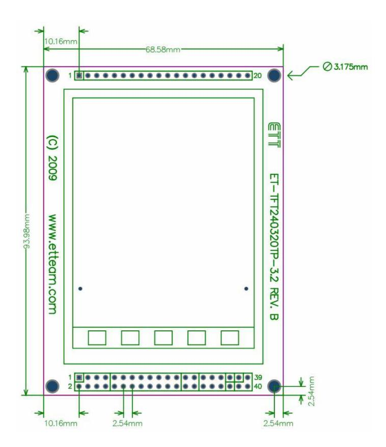
Figure 6.2 Displays size of Board ET-TFT240320TP-3.2 REV.B.
