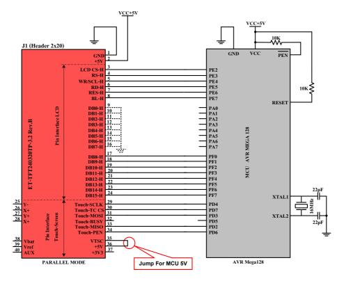
Figure 3.2B displays example of connecting Board ET-TFT240320TP-3.2 REV.B with MCU AVR #Mega128(5V).
