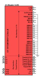
Figure 3.1D Displays how to connect Pin Interface LCD that is not used as identified with the dotted line above.
