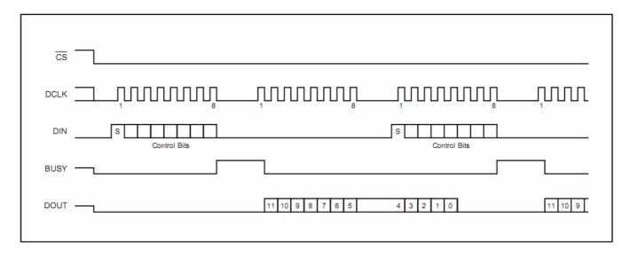
Figure 4.2.3 displays Conversion Timing Diagram, 16 Clock-per-Conversion, 8bit bus Interface.
