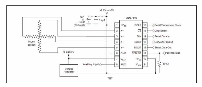
Figure 4.2.1 display how to connect circuit of Touch Screen and ADS7846.
