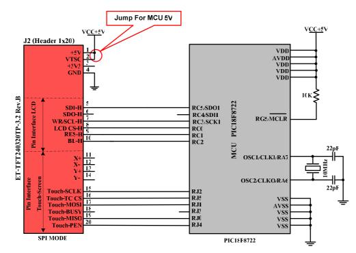
Picture 3.1C Displays example of interfacing Board ET-TFT240320TP-3.2 REV.B with MCU PIC #18F8722(5V).
