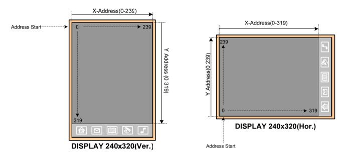
Figure 6.1 displays how to refer address position on LCD Display that is horizontal and vertical lines.
