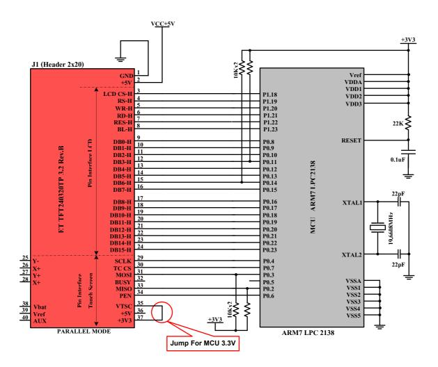
Figure 3.3A displays example of connecting Board ET-TFT240320TP-3.2 REV.B with MCU ARM7 #LPC2138(3.3V).
