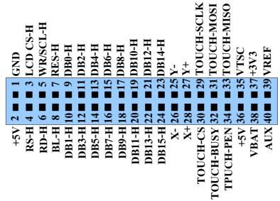
Figure 2.3 displays pin position of Header 2x20(Parallel-Mode:8,16 Bit)(front view as shown in the figure 2.1 (A)).
