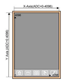
Figure 4.2.2 displays area of Touch Screen and the ADS value that has occurred on the line of X and Y axis.
